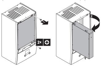
**4** If you have to do work behind the user interface panel or upload new software into the user interface, open the user interface panel.
