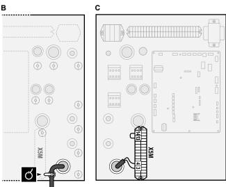
**3** Connect the high voltage wiring as follows:
