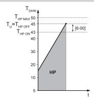
Heat pump. If heating up time by the heat pump takes too long, auxiliary heating by the backup heater can take place
