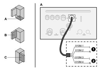
High voltage Smart Grid contact 1High voltage Smart Grid contact 2
