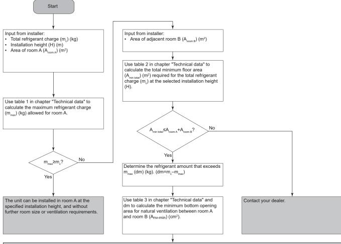
Unit can be installed in **room A** if you provide 2 openings (one at the bottom, one at the top) between room A and B to ensure natural ventilation. The openings must comply with the following conditions:
