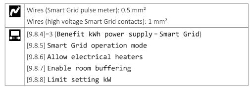
The wiring of the Smart Grid in case of high voltage contacts is as follows:
