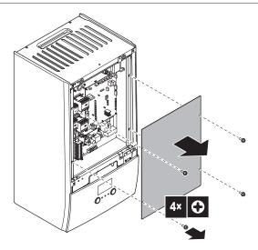
**3** If you have to do work behind the switch box, open the switch box.
