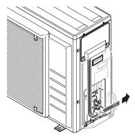
7 Connect an earth leakage circuit breaker and fuse to the power supply line.
