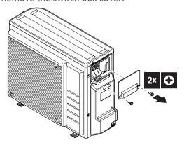
2 Remove the refrigerant piping cover.
