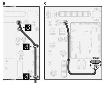
**4** Fix the cables with cable ties to the cable tie mountings. If necessary, bundle excessive cable length with a cable tie.
