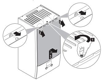
2 If you have to connect electrical wiring, remove the switch box cover.
