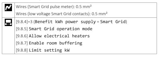
The wiring of the Smart Grid in case of low voltage contacts is as follows:
