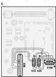
2 Connect the low voltage wiring as follows:
